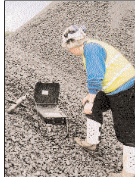
Figure 7. The ash probe in use.
